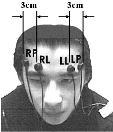
Figure 1 Schema of NIRS measurement. Near infrared emitters with light emitting diodes (LED) were positioned on the frontal scalp's upper orbits; right LED (RL) and left LED (LL) were set. Detectors with photo diodes were positioned 3 cm lateral from the respective LEDs; right photo diode (RP) and left photo diode (LP) were set.
